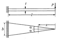
0.52 The area moment of inertia about the neutral axis of a cross-section at a distance x measured from the free end is
