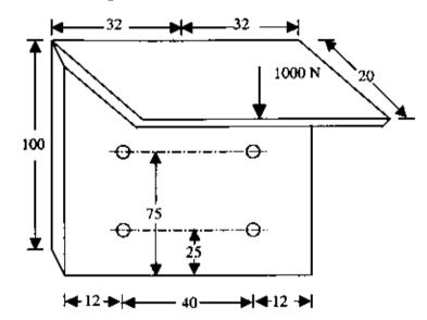
Direct shear stress (in MPa) in the most heavily loaded rivet is
