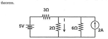
Find current "I" flowing through  $2\Omega$  in given circuit by using superposition
