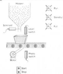
This process requires that boxes moving on a conveyor be automatically positioned and filled. The sequence of operation for the continuous filling operation is as follows:
